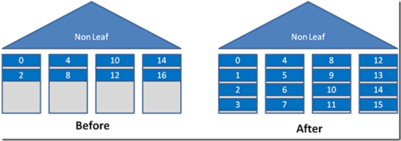
Figure 3: A fully logged insert under trace flag 610
